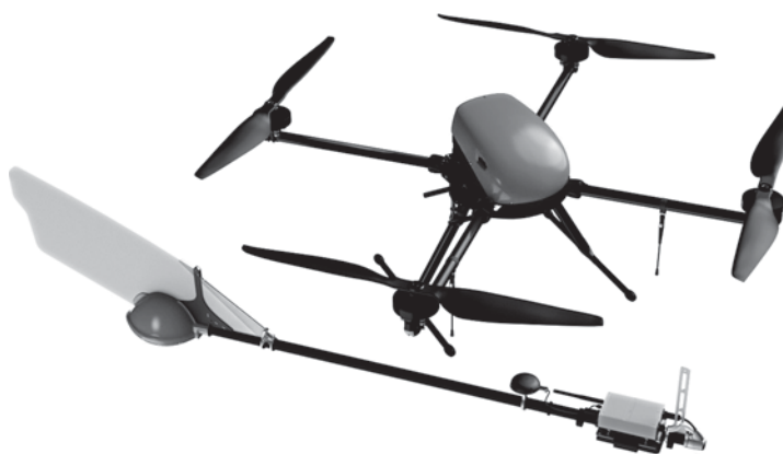
Fig. 4. Geoscan 401 Geophysics complex for high-precision aeromagnetic survey.
