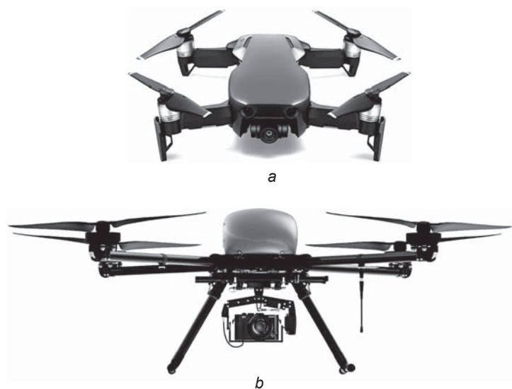
Fig. 3. Unmanned aerial vehicles used for aerial photography. a – mini drone DJI Mavic Air (China); b – Geoscan 401 (Russia).
