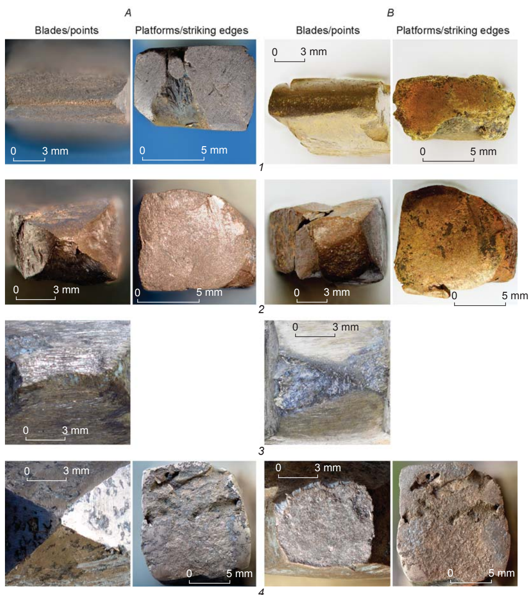
Fig. 4. Active parts of experimental bronze tools after manufacture (A) and after use (B). 1, 3, 4 – 7–8 % tin bronze; 2 – 4–5 % tin bronze. 1 – chisel; 2 – pointed tool; 3 – spear-shaped chisel; 4 – battle axe.
