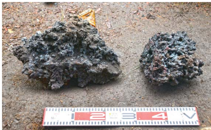
Fig. 7. Monolith of a conglomerate with inclusions of bloomery iron. Experiment of 2017 by the author.
