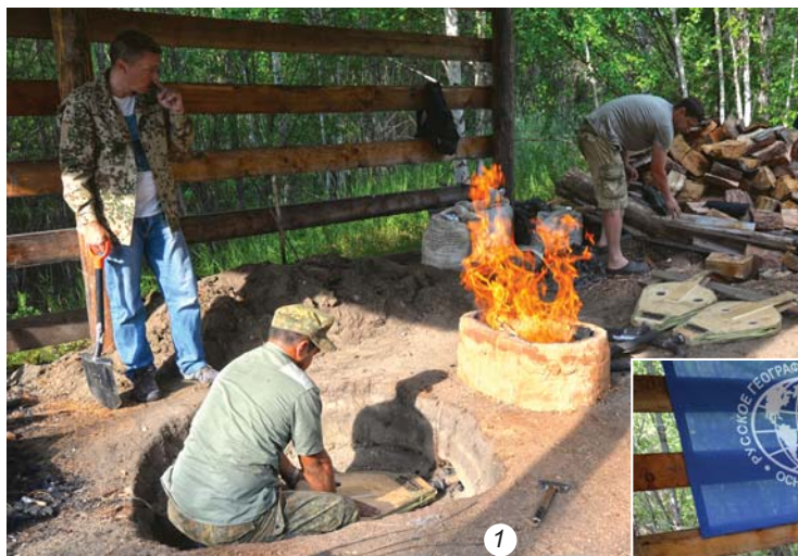
Fig. 6. Processes of warming up the furnace (1), loading furnace charge (2) and upper air-blasting (3). Experiment of 2017 by the author.
