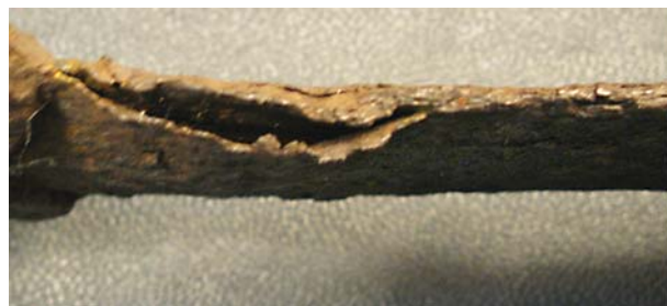
Fig. 2. Damage-signs on blades (packs of exfoliated plates) of Klyuchi (1) and Novoobinka (2) swords.
