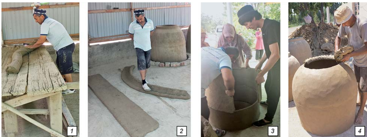
Fig. 4. Making tandoors using large-diameter coils. Photo by N. Petrova.
