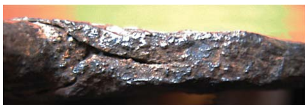
Fig. 4. Forge-welds adjusting guard to grip on Klyuchi (1, 2) and Novoobinka (3) swords.
